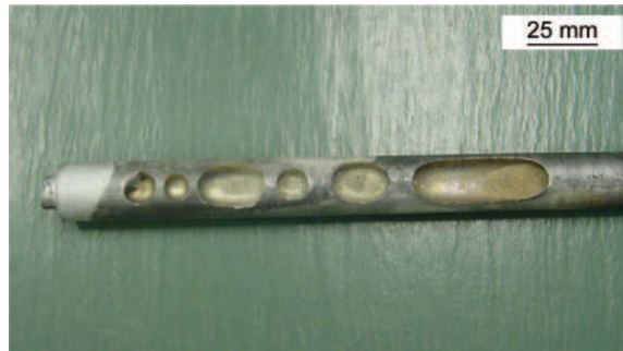
Fig. 7.19 The AZ91 alloy, solidified within a nozzle with surface bubbles formed by magnesium vapor
