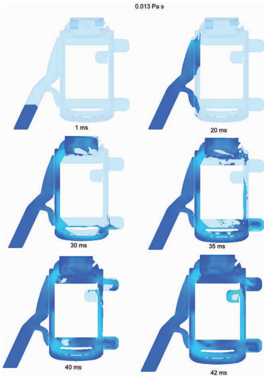
Fig. 2.8 The FLOW-3D simulation of filling a cavity of cell phone housing with a weight of 5.3 g using magnesium alloy Mg-9Al-1Zn with a viscosity of 0.013 Pa s
