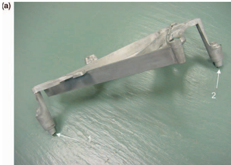
Fig. 5.28 The application of hot runners in magnesium molding: a an automotive bracket injected from two directions through cold sprues and cold runners
