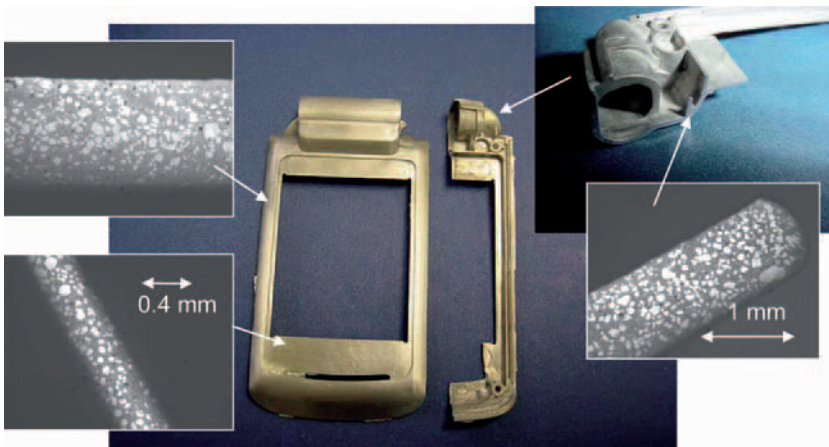
Fig. 9.24 The distribution of solid content within the thin-wall component of small size, injection molded using solid content with an average of 35%
