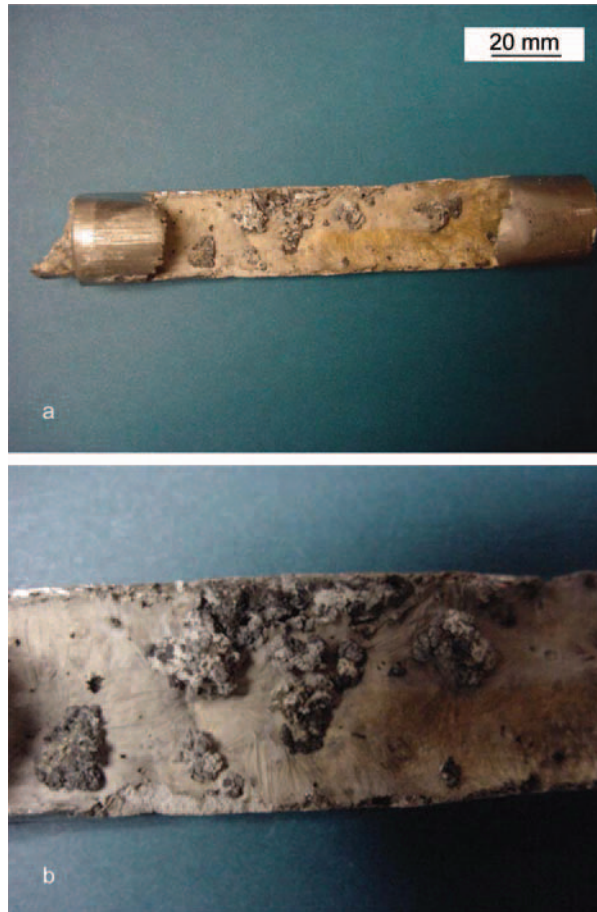
Fig. 7.20 The formation of oxide on the free surface of molten magnesium alloy within the machine nozzle
