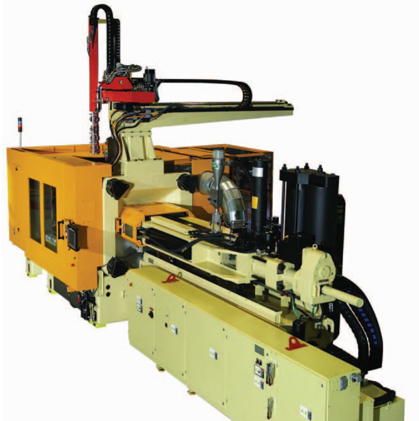
Fig. 3.2 The HyMet™ magnesium molding machine with a clamp force of 500 tonnes
