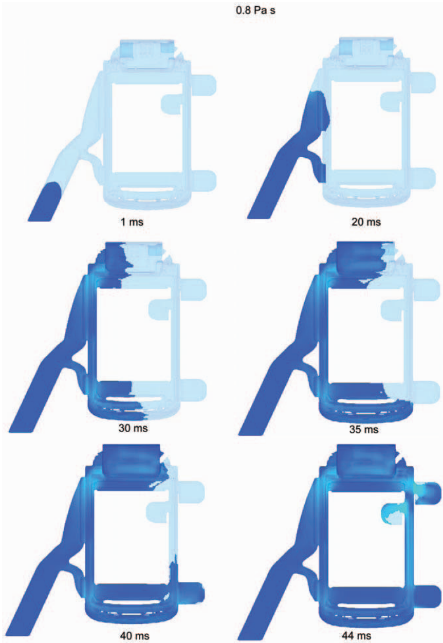
Fig. 2.9 The FLOW-3D simulation of filling a cavity of cell phone housing with a weight of 5.3 g using magnesium alloy AZ91D with a viscosity of 0.8 Pa s
