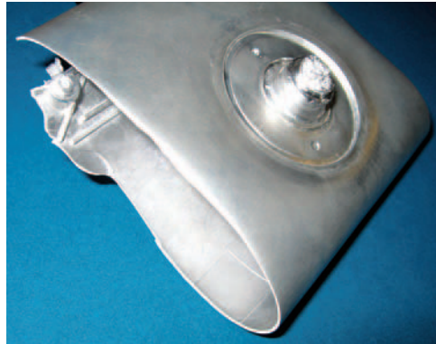
Fig. 12.16 The 180 deg bending test of a component with a wall thickness of 0.7 mm showing a superior ductility after NLM (Mg-9Al-1Zn)
