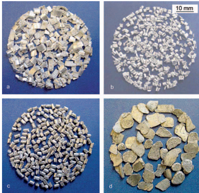
Fig. 6.5 Non-conventional morphologies of particulates: a F1-MEZ flakes obtained by mechanical fragmentation of an ingot; b F2-AZ91 flakes; c P1-AZ91D pellets obtained by a combination of solid state extrusion and cutting; d R1-AZ91D recycled feedstock generated from fragmentation of die-cast components
