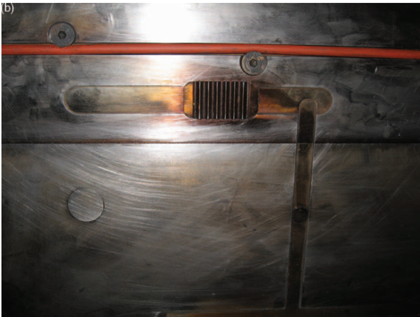
Fig. 3.24 The concept a and practical implementation b of the static vacuum valve based on chill blocks
