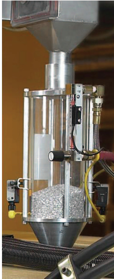
Fig. 3.15 The feeder used to supply the chipped feedstock to the injection molding machine
