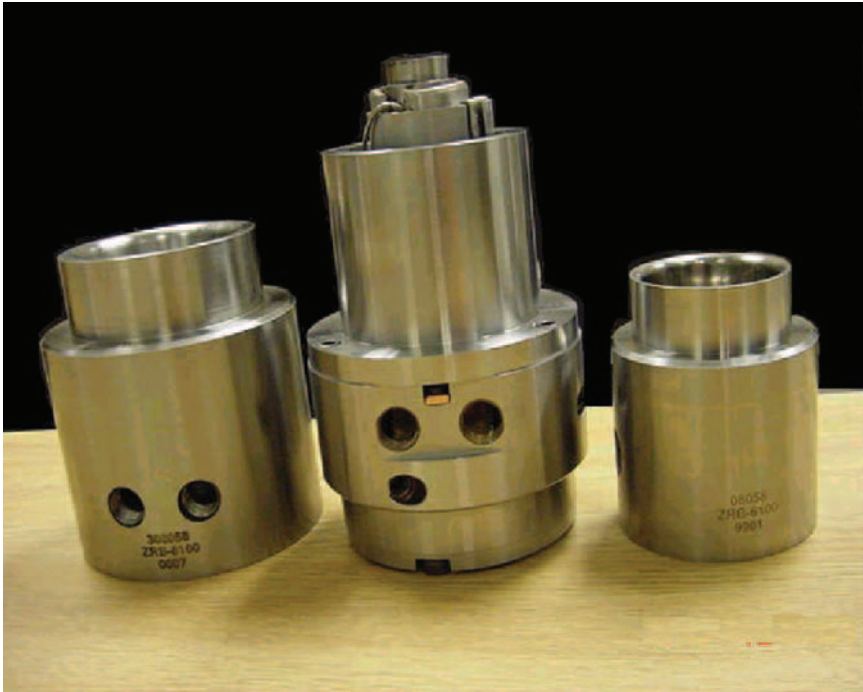
Fig. 3.20 The typical cold sprue inserts used in die casting along with the hot sprue solution for magnesium molding (shown in the center)
